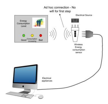
The target of this gadget is to avoid that a device could lose its efficiency due to aging and invisible faults. For example a three years old washing machine can lose up to 40% of its efficiency due to bad maintenance. The gadget allows us to check and monitor more critical devices all along their life, showing a clear indication of the equipment status and also it could be a motivation for all us.
